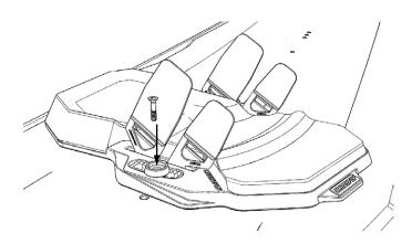
**5.** Put 2 pcs Hexa washers in place, one to the left and the other one to the right side of the Hexa footpad. Make sure the holes in the washer are aligned with the inserts on the board. Tighten 2 pcs screws slightly - left and right side of the Hexa footpad.
