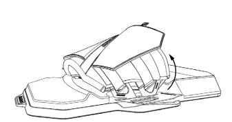
**9.** Slide the Quattro Stix inside the footstrap. Slightly tighten and close the threaded velcros. Leave the velcros a bit loose and close the top velcro. Leaving the velcro loose will make threading the velcro on the other side of the footpad easier.
