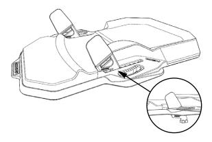
**1.** Take 1 pc Quattro Stix Short and 1 pc Hexa footpad Right. Place the Quattro Stix Short in the front position of the Hexa footpad frame on the left and on the right side.
