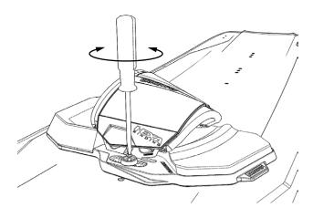
**14.** If further adjustments for the angle of the binding is needed, loosen the screws a little until the Hexa Binding is able to spin. Adjust the angle again to the desired position and fully tighten the screws.
