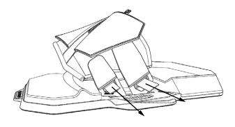
**8.** Take the Hexa footstrap Right and open the velcro. Thread the velcro through the Quattro Stix. It is best to start on the Quattro Stix Long in the left side of the Hexa footpad right (inside of the foot). Then continue with threading the velcro through the Quattro Stix Short on the same side.
