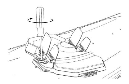
**7.** Fully tighten the screws. Please check the footpad screws after the first few rides, as they may come loose. If loose, make sure to fully tighten the screws.
