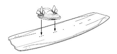
**4.** Place the Hexa footpad Right on the board and select desired insert position. This determines your stance width.
