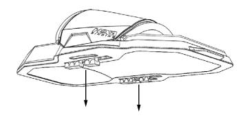
**15.** If further adjustments for the footstrap position and footpad position are needed, undo the screws completely. Lift up the Hexa Binding, push the Quttro Stix down so they pop out of the Fusion Frame. Adjust the Quattro Stix to the desired position and pop them back in the Fusion Frame. Mount the Hexa Binding back on the board to the desired position and fully tighten your screws.
