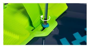
**6.** Fully tighten the screws. Please check the footpad screws after the first few rides, as they may come loose. If loose, make sure to fully tighten the screws.
