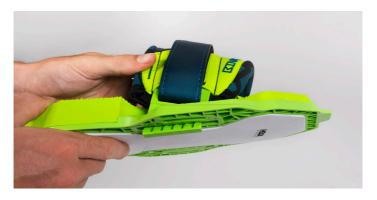
12. If further adjustments for the footstrap position and footpad position are needed, undo the screws completely. Lift up the Binary Binding, push the Binary Stix down so they pop out of the footpad Frame. Adjust the Binary Stix to the desired position and pop them back in the footpad Frame. Mount the Binary Binding back on the board to the desired position and fully tighten your screws.
